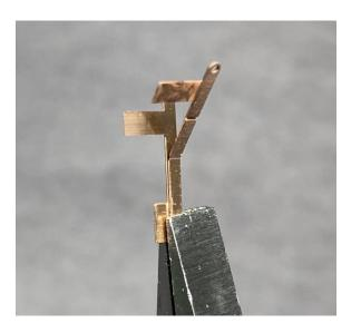
After the two halves of the center stanchion are folded back onto themselves I bend the horizontal arm of the stanchion down until it is perpendicular to the center stanchion. In the photo there is a small rectangular piece at the base of the stanchion right where the pliers are holding the stanchion. This will be folded back over the stanchion next.
