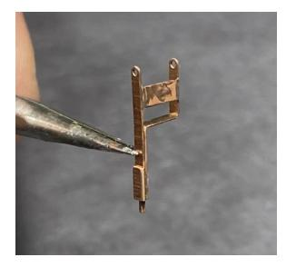
I then fold the flap on the center stanchion over so that it is resting on the other flap. I use CA to attach these flaps.
