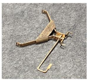
The pilot grab rails are in to sections. This is done since a fully formed grab rail would not be able to be threaded through the two holes in the center of the handrail stanchions. Thread the straight end of the grab rail through one of the holes in the stanchion. A little CA is useful for holding it in place. When the grab rail is firmly in place add the second on the other side of the stanchion. Again, a small drop of CA will hold the grab rail firmly in place.
