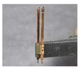
Once both face plates are bent back against the stanchion I fold the two stanchions back. They should end up being perpendicular to the square piece of metal that joins the two stanchions at the base.
