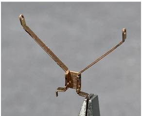
The MU receptacle mounting plate is an optional piece. Locomotives that were not MU equipped might not have this piece although some did. Check with prototype photos to determine if it is needed on your model. Fold each end so that it is perpendicular to the center trapezoidal piece of metal.
