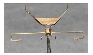
The finished handrail assembly is ready for installation on the model. If you chose to do so you can add the wire handrail to the stanchion prior to installation on the model. I recommend .015" phosphor bronze wire for this. I do find it easier to bend the handrails on the model sometimes.
