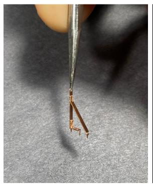
The bottom of the angled brace has a fold line and a pin. The bottom is folded to be parallel to the stanchion.
