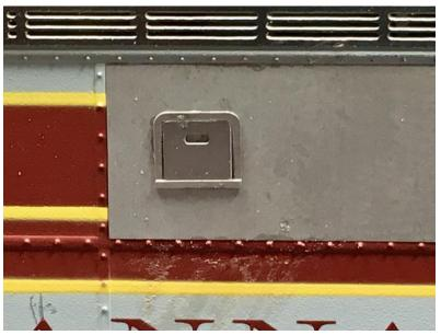
This is a sand fill hatch that has been properly assembled and installed. The outside rim should like an upside down "U". The decorative etch line is at the bottom of the sand fill hatch. CA is used to attach the hatch to the sides of the locomotive.
