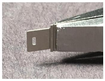
This photo shows the sand fill hatch held in a pair of flat nosed pliers. Note that the hatch is being held just below the fold line. The other etch line is the decorative line that was mentioned above.
