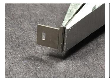
Fold the top portion of the sand fill hatch backward. This will leave the decorative etch line exposed. If you fold the sand fill hatch incorrectly this decorative etched line will disappear.
