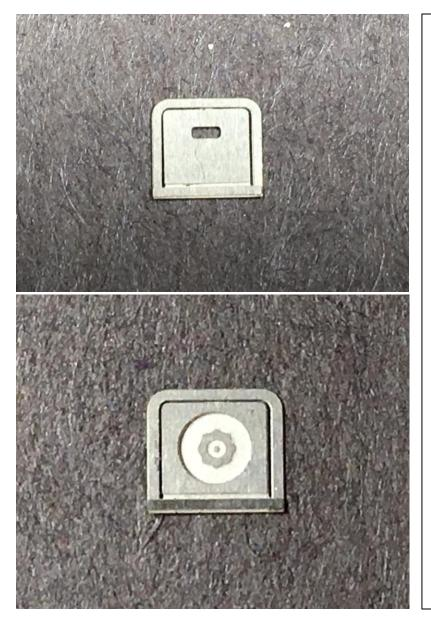
When folded correctly this is how the two sand fill hatches should look. Note that the decorative fold line we keep referring to is noticeable across the lower portion of the fill hatch. The fold line is at the extreme bottom edge of the part.
