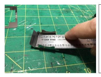
Step 2. Fold the fuel tank extension sides up starting at the fold line closes to the center of the tank. Those folds should match the ends of the fuel tank extension. A metal edge such as this scale will help greatly when bending the at the folds. The metal edge will allow you to bend only that particular bend line when used in this manner.
