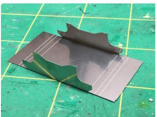
Step 1. Fold the fuel tank extension ends up. Note that the fold lines will be INSIDE the tank extension.
