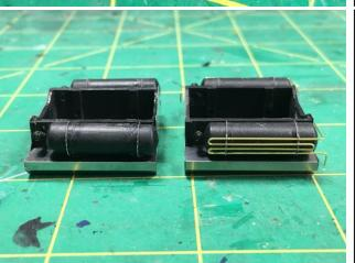
Step 9. Mount the main reservoir tanks to the fuel tank. CA on the back pads of the mounting bracket should do fine. This is important. Make sure that you install the correct tank on the correct side. One tank has 5 rows of pipes while the other has 4 rows. The Engineer side should have 4 rows while the Fireman Side should have 5 rows.
