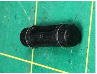
Step 8a. Note the location of the pipe brackets. They should be in the front of the tank opposite the mounting pad. If your pipe brackets are anywhere but this location try again.
