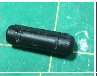
Step 7. Prepare the main reservoir tanks for installation of the Main Reservoir Mounting Brackets. The brackets are slid over each end of the reservoir tanks up to the straps molded into the tank. In order to do this some material needs to be removed from the reservoir tank mounting pad on the back of the tank. The photo shows two cuts made into the pad with a razor saw lining up with the outer edge of the molded straps.
