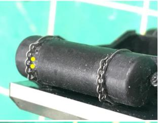
Step 11. Do the same for the Fireman Side or the 5 pipe side. Note that the drilling location for the holes is different on this side. The holes will be closer together. The bracket in the foreground has the pipe bracket top half installed so you can see how they will work when pressed into the mounting holes.
