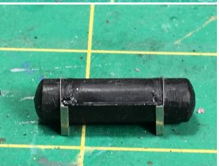
Step 8. Remove the excess mounting pad material with a file, knife or sanding stick. When that is done fold the mounting plates of the mounting brackets and slide the brackets over the tank ends. Secure the brackets to the rear of the mounting pad using CA. It is fine if the brackets slide around a bit on the front of the tank as they are not secured with CA at this time. Try to line them up the best you can.
