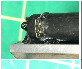
Step 10. In order to install the Pipe Bracket Top Half sections two mounting holes have to be drilled. I drill them on the inside edge of the bracket, into the molded strap. A #80 bit is the smallest hole you can drill and still have the mounting tabs work. Drill the holes in the location of the yellow dots in the photo. Do this for both brackets. Note that this is the 4 pipe side or the Engineer Side.
