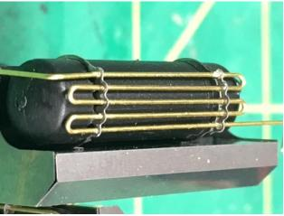
Step 12. Bend and install the piping. I used .015" brass rod for this as it bends easily and is durable. The bent piping assembly will be flat until it is mounted into the divots on the pipe brackets. The pipe bracket top halves will pull the piping inward toward the tank matching the curvature of the tank. A little CA along the mating surfaces of the bracket halves as well as on the mounting pins should hold everything together.
